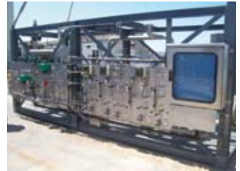
A WELL-EQUIPPED PLANT. The pilot plant consist of the following subsystems: sea water pumping and filtering; sea water flow and pressure control; gases storage, treatment and dosage; reactor-dissolver; PH-meters, sample takers and other systems to assess the achieved degree of dissolution. Taking into account the data obtained by this systems to date, the tests performed have shown satisfactory results but still some parameters are under study in order to obtain optimum operation configuration.
