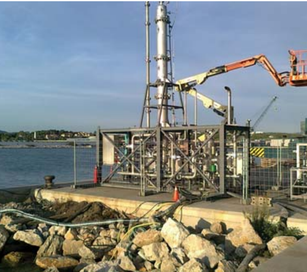
A WELL-EQUIPPED PLANT. The pilot plant consist of the following subsystems: sea water pumping and filtering; sea water flow and pressure control; gases storage, treatment and dosage; reactor-dissolver; PH-meters, sample takers and other systems to assess the achieved degree of dissolution. Taking into account the data obtained by this systems to date, the tests performed have shown satisfactory results but still some parameters are under study in order to obtain optimum operation configuration.
